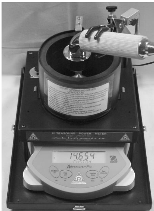
Front view of the UPM-DT-1&10AV. Shown is the electronic balance, base assembly, and test tank.
