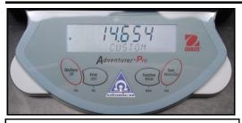
UPM-DT Series Ultrasound Power Meters feature a high contrast alphanumeric LCD display. Membrane "touch buttons" enable quick setup, automatic zero, selection of units for the power reading (grams or Watts "custom"), and printer control.
