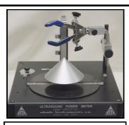
The cone target and transducer positioner. (Tank not shown.)
